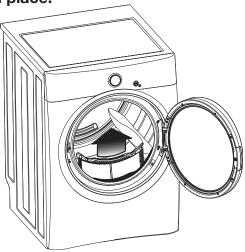
A clean lint filter allows the dryer to operate more efficiently.
