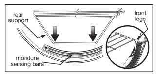
Place items to be dried on top of the rack, leaving space between items and not allowing them to hang over the sides or through the holes. The weight should not exceed 10 lbs (4.5 kg). Select the **air** (no heat) setting for items containing plastic, foam rubber, rubber-like materials, feathers or down.
